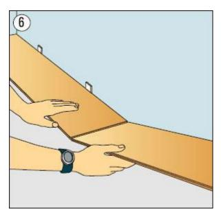
**STEP 6** Position the second panel with its tongue side at an angle against to the groove of the first panel already in place. Slightly push in and bring down the second panel to connect these two panels. Repeat these steps to complete the first row.
