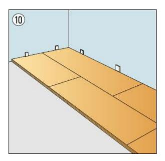
**STEP 10** Slightly push in and bring the panels until fully flat down. Panels in adjoining rows must be off-set at least 12" minimum. Do not make the first panel of each the same length.
