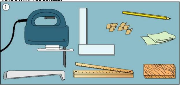
**STEP 1 -** General tools needed are pencil, measuring tape, square ruler, whip saw or a fretsaw and a number of wedges or spacers.
