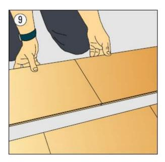
**STEP 9** Tilt the panels together and position the tongues into the grooves of the previous row at an angle.
