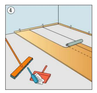
**STEP 4 -** When the sub floor had been prepared accordingly, lay the P.E. sheets and the P.E. foams underlay for the next 5~10 rows of panes that you will install.
