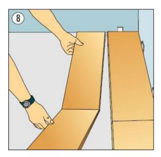
**STEP 8** Apply the same methods as the first row to join the panels of the second row.
