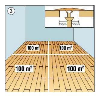
**STEP 3 -** If the install areas are more than 100m2, it is recommended to use suitable profiles to separate the floors. This is also applicable if laying the flooring over several rooms, even though the room sizes may be less.
