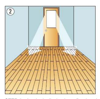
**STEP 2 -** Aesthetically, laminate flooring should be laid parallel to the direction of the incoming light. This helps to diminish the appearance of long seam between panels. Lay in the longitudinal direction in a long and narrow room.
