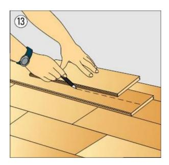
**STEP 13** For the final row, if the wall is not straight, adapt the panel to the course of the wall by using a small piece (as a rule), place it on top of the cull panel. Use a pencil to mark on the full panel and cut according to the marking line, with the consideration of sufficient expansion gap.
