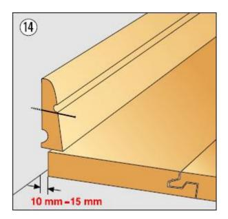
**STEP 14** Remove all spacers, install the skirting and profiles. Do not fasten them on the laminate flooring. A durable elastic substance can be used to seal gaps.
