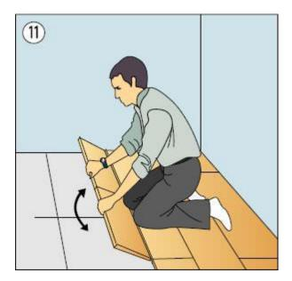
**STEP 11** As of the 4th row onwards, apply the same method as 2nd and 3rd row but position yourself on the flooring which had been installed.
