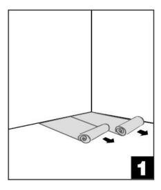
STEP 1 - Prepare Floor. Underlay on the dry and levelled subfloor
