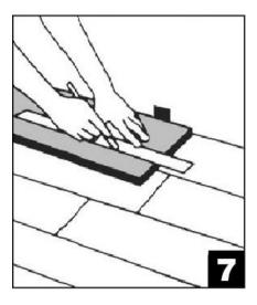
STEP 7 - To fit the final row, lay a plank upside down on the flooring as per diagram with the tongue side close to wall. Take another plank and place it right on top of the previous row and use it as a ruler. Don't forget to allow room for spacers. Cut the plank and attach into position.
