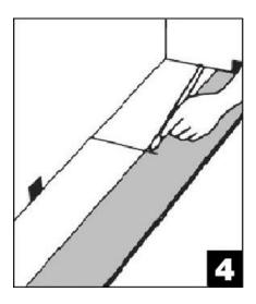
STEP 4 - For the last plank of a row, flip a full plank to its under-side and place beside the row. Measure and mark the required length. Use a ruler and utility knife to score the plank and snap off. Insert as previous 3 diagrams.
