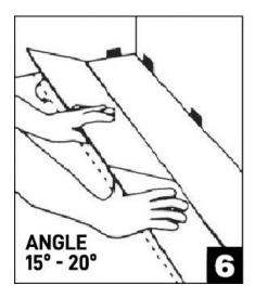
STEP 6 - To start second row, assemble your entire row on the subfloor before attaching it to the first row. To attach, tilt and push the side tongue into the side groove of the first row at an angle of 15° to 20°. Lower and click into place lining the edges up carefully. Continue laying remaining planks in this matter.
