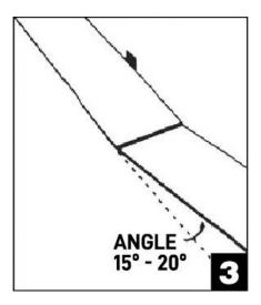
STEP 3 - Insert 2nd plank's end tongue to 1st plank's end groove at an angle of 15° to 20°. The plank will click into place when lowered. Line up edges carefully. Planks should be flat to the floor.
