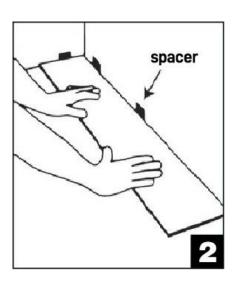
STEP 2 - Start at a corner. Place first plank with tongue side facing wall. Use spacers to maintain an expansion space of 8mm between wall and flooring.
