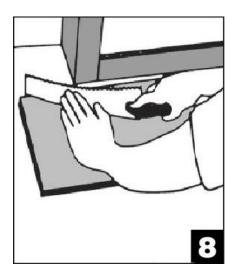
STEP 8 - The gap between the bottom of a door and the SPC flooring should be 1 cm height. To trim door frames, turn a plank upside down. Place it next to the door frame as per diagram. Use a handsaw and cut away the necessary height so that the planks can slide easily underneath the frame.
