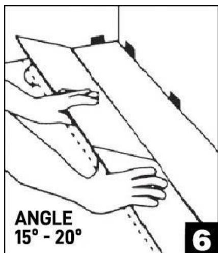
**STEP 6 - To start second row, assemble your entire row on the subfloor before attaching it to the first row. To attach, tilt and push the side tongue into the side groove of the first row at an angle of 15° to 20°. Lower and click into place lining the edges up carefully. Continue laying remaining planks in this manner.**
