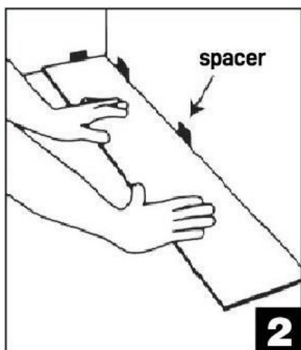
**STEP 2 - Start at a corner. Place first plank with tongue side facing wall. Use spacers to maintain an expansion space of 8mm between wall and flooring.**
